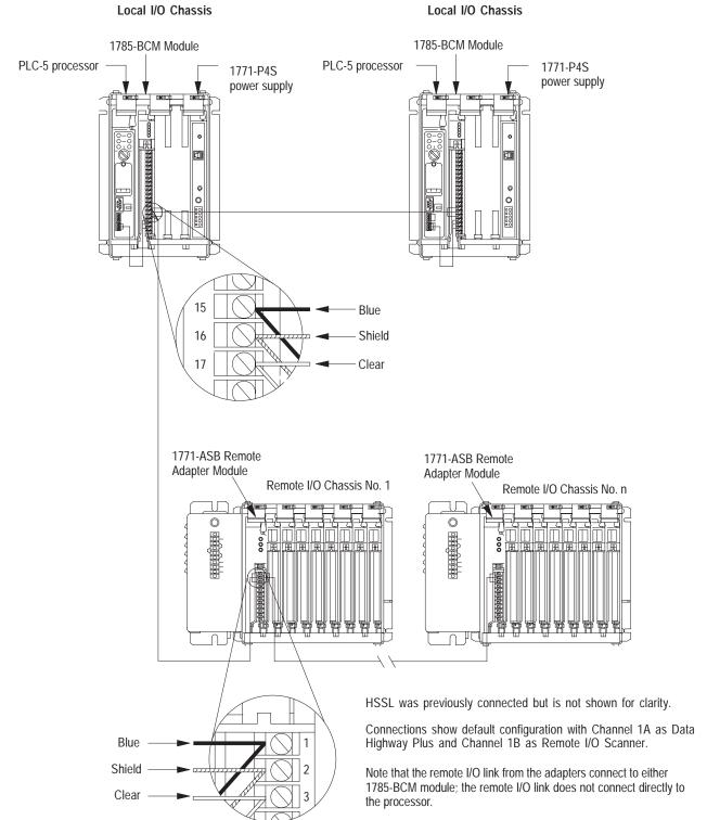
**6.** Connect the other end of the 1770-CD cable to terminals **1, 2, and 3** on the wiring arm of the Re mote I/O Adaptor module as shown in Figure 3.10.
