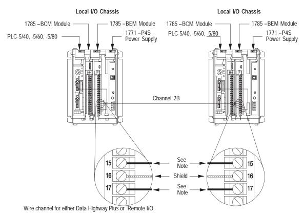
Data Highway Plus – connect the signal conductors with Clear, Shield, and Blue insulation to terminals 15, 16, and 17 of 1785 – BEM module, respectively.
