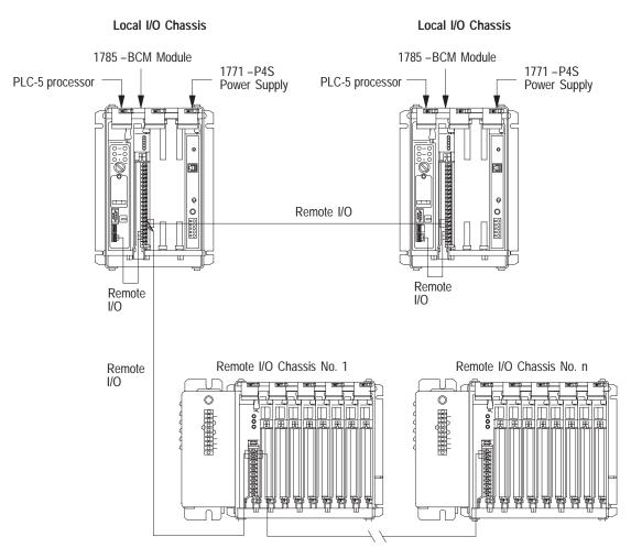
Connections show default configuration with Channel 1A as Data Highway Plus and Channel 1B as Remote I/O Scanner.
