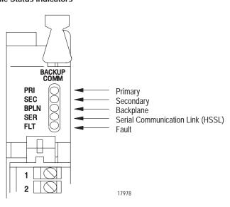
All indicators light at power up or when a hardware fault occurs in the 1785-BCM module. With the exception of the FLT indicator, all of the 1785-BCM module's indicators are related to individual bits of the system status word. For more information on the system status word, refer to Chapter 5, "Operating Your PLC-5 Backup System."
