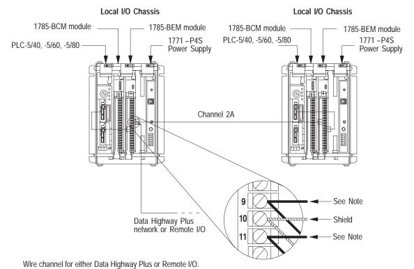
Data Highway Plus – connect the signal conductors with Clear, Shield, and Blue insulation to terminals 9, 10, and 11 of 1785 –BEM modules respectively.
