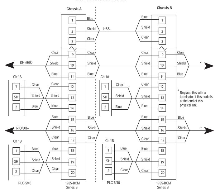
Figure 3.5 1785-BCM Module Connections
