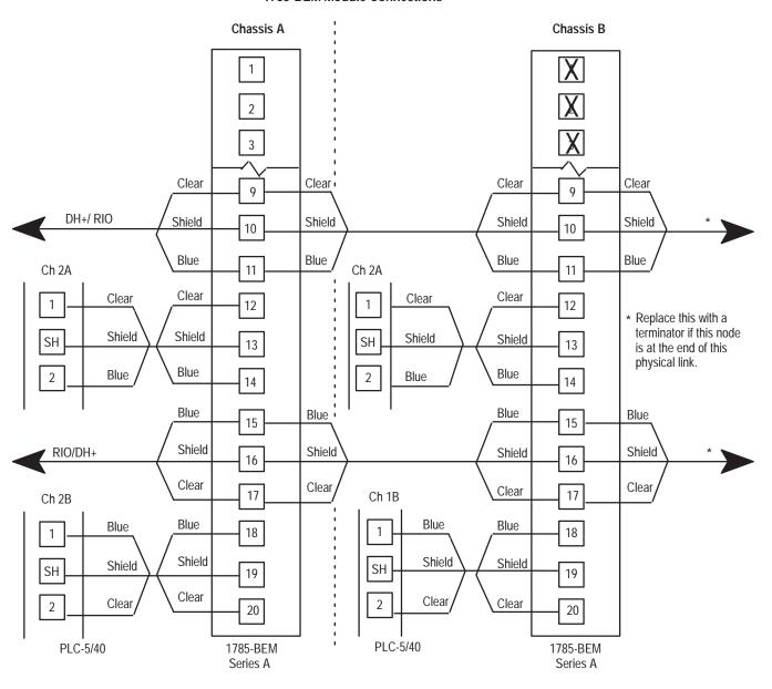
Figure 4.7 1785-BEM Module Connections
