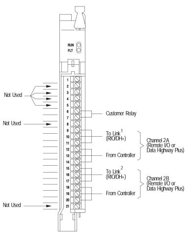
Terminals 9, 10, and 11 are connected between the 1785 –BEM modules in the backup system; in addition terminals 9, 10, and 11 of one of the 1785 –BEM modules are connected to the DH+ network or to the Remote I/O link.
