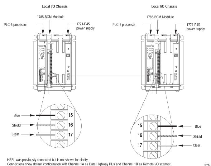
**5.** Connect one end of a 1770-CD cable to terminals **15, 16, and 17** on the wiring arm of one of the 1785-BCM modules as shown in Figure 3.10.
