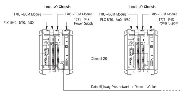
1785-BCM module was connected in Chapter 3 but is not shown for clarity. Also, 1785-BEM module Channel 2A was previously connected but is not shown for clarity.
