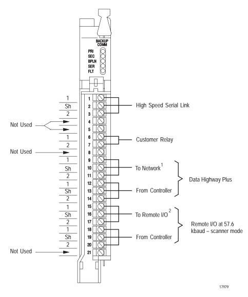
Figure C.1 1785-BCM Series A Module Communication Links
