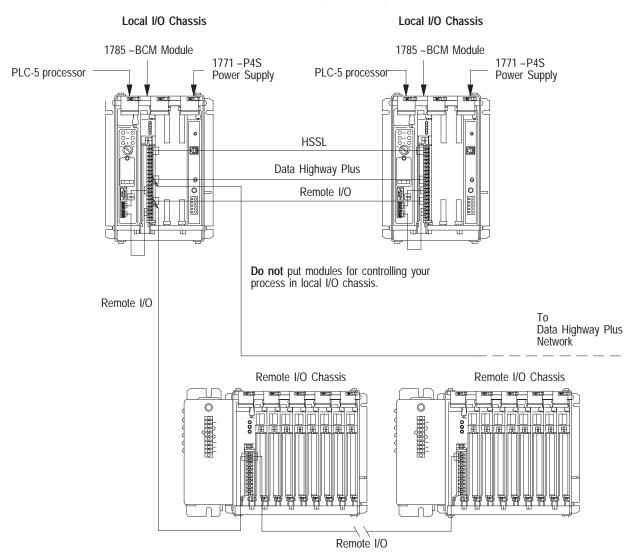
Some applications that use more than two ports (PLC-5/40, PLC-5/60, or PLC-5/80 processors) may require a 1785-BEM module (not shown).
