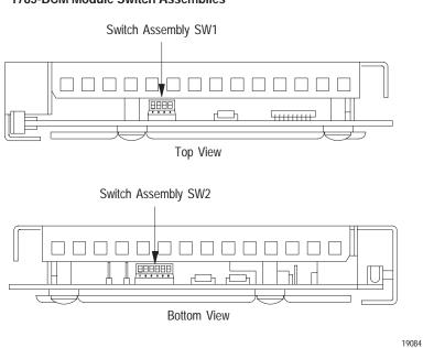
Table 2.C 1785-BCM Module Switch Assembly Functions
