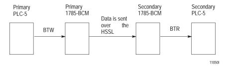
For detailed information about data transfer from the primary to the secondary system, refer to Chapter 5, "Operating Your PLC-5 Backup System."
