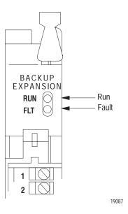
**RUN** (green) indicator is on to show normal operation of the 1785-BEM module.
