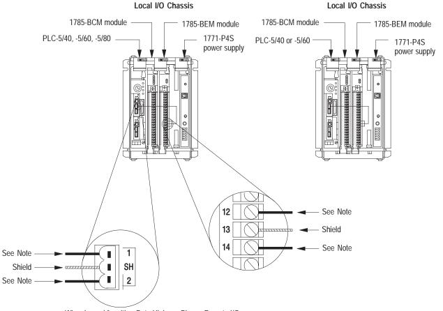
Wire channel for either Data Highway Plus or Remote I/O.
